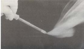
Figure 14: Air current tubes
