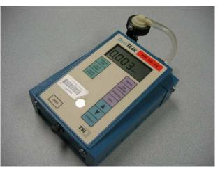
Figure 10: DustTrak<sup>™</sup> fitted with cyclone elutriator for static monitoring and checking of dust controls
