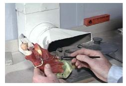
Figure 13A: Fixed exterior hood (HSE UK)
